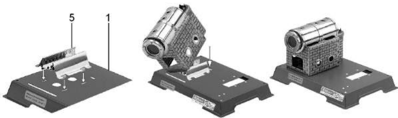
Fig.2.2.2: mounting the burner slide and the boiler house
