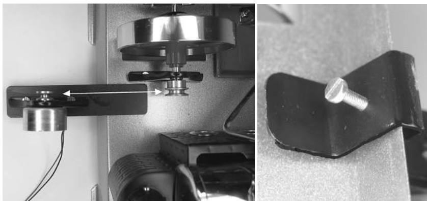
Fig.3.27: Assembling of the generator: a) both pulley wheels in one line, b) compression fitting, underneath the basic plate
