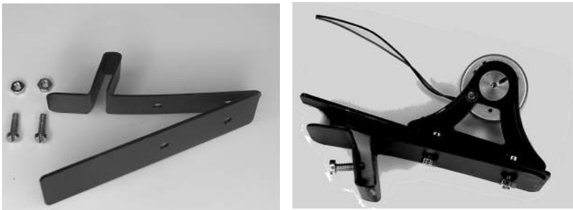
Fig.3.26: Parts for mounting the generator, a) two-piece holder of the generator, b) mounting support of the generator and adjusting screw
