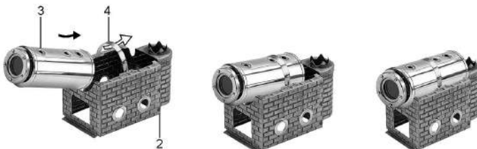
Fig. 2.2.1: mounting the boiler
