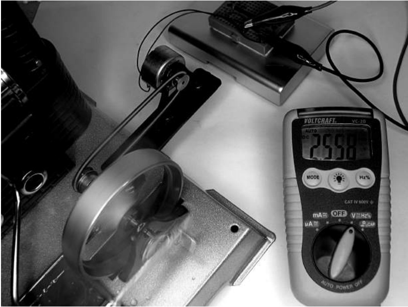
Fig.3.29: measuring the voltage of the generator with a multimeter
