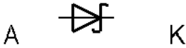
Fig.3.13: circuit symbol, Schottkydiode, the left side signed with A is the anode (+), the right side signed with K is the cathode (-)
